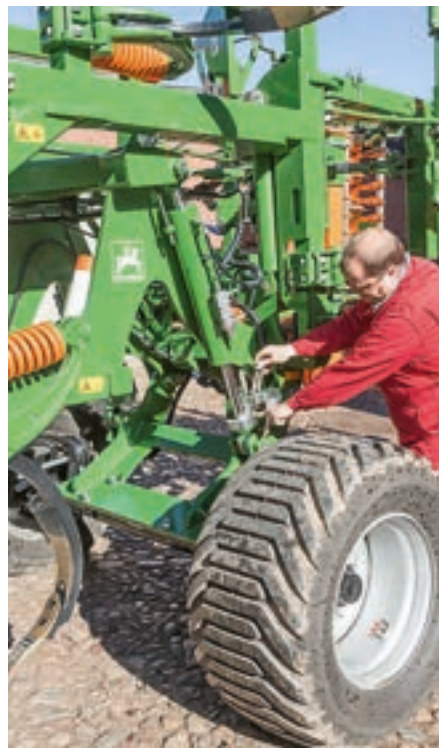
When the rear roller is not in use, the working depth is set by fitting stops to the running gear.
