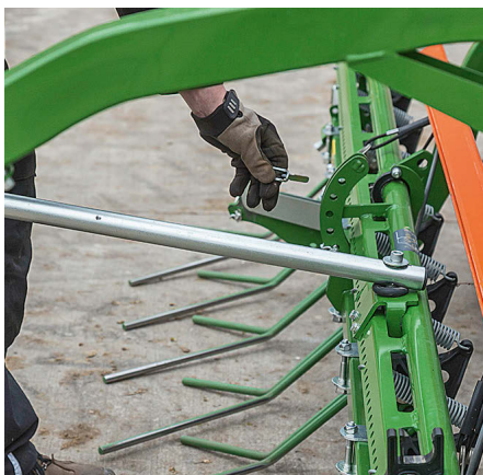
The robust 15mm following harrow tines are straightforward to alter for good seed covering.
