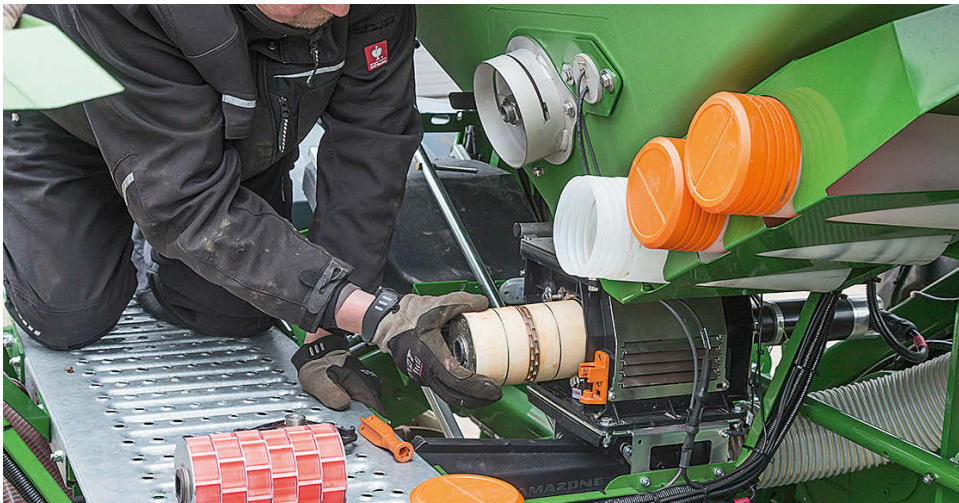
The metering units are stored in capped plastic tubes and are swapped in no time (left pic).
