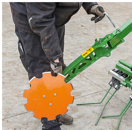
Another nice touch: the pre-emergence markers are easily adjusted to different track widths.
