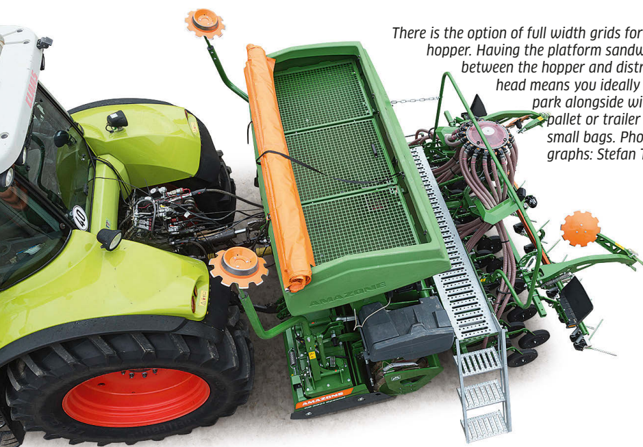
The sensor on the top link switches the Centaya drill on the headland and controls tramlining.
