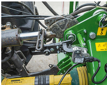
The sensor on the top link switches the Centaya drill on the headland and controls tramlining.
