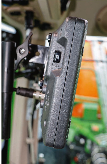
A USB slot on the terminal is equipped with a Wi-Fi adapter that links to the tablet.
