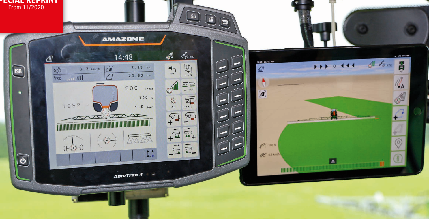
The AmaTron TwinApp interface is opened on the iPad (the screen on the right) to show the field view. The AmaTron 4 terminal is looking after the sprayer functions.
