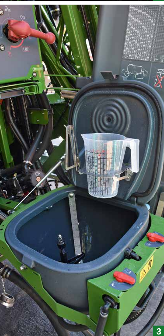
◁ 1) Coupling and uncoupling the sprayer is easy. 2) The uncluttered operator control panel. 3) The 60-litre inductor hopper comes with a measuring cup and further useful details.
